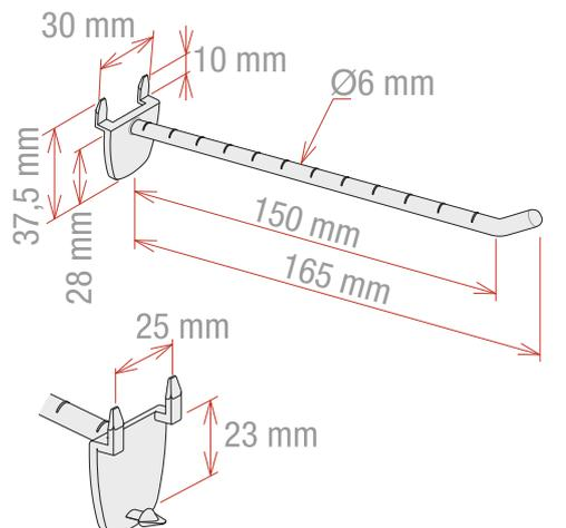
Display hook with 3 back rear tips that allow automatic insertion without previous die cut.
