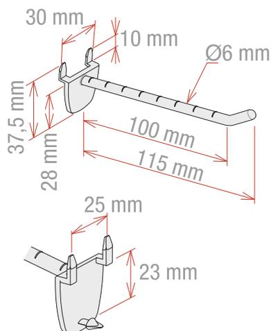
Display hook with 3 back rear tips that allow automatic insertion without previous die cut.
