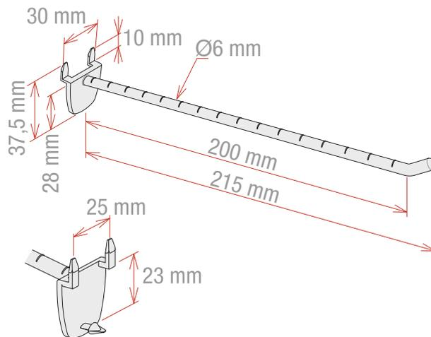
Display hook with 3 back rear tips that allow automatic insertion without previous die cut.
