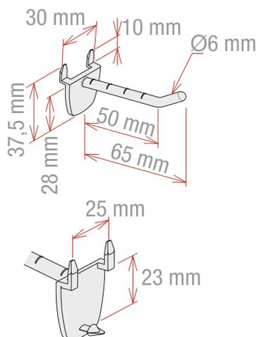
Display hook with 3 back rear tips that allow automatic insertion without previous die cut.
